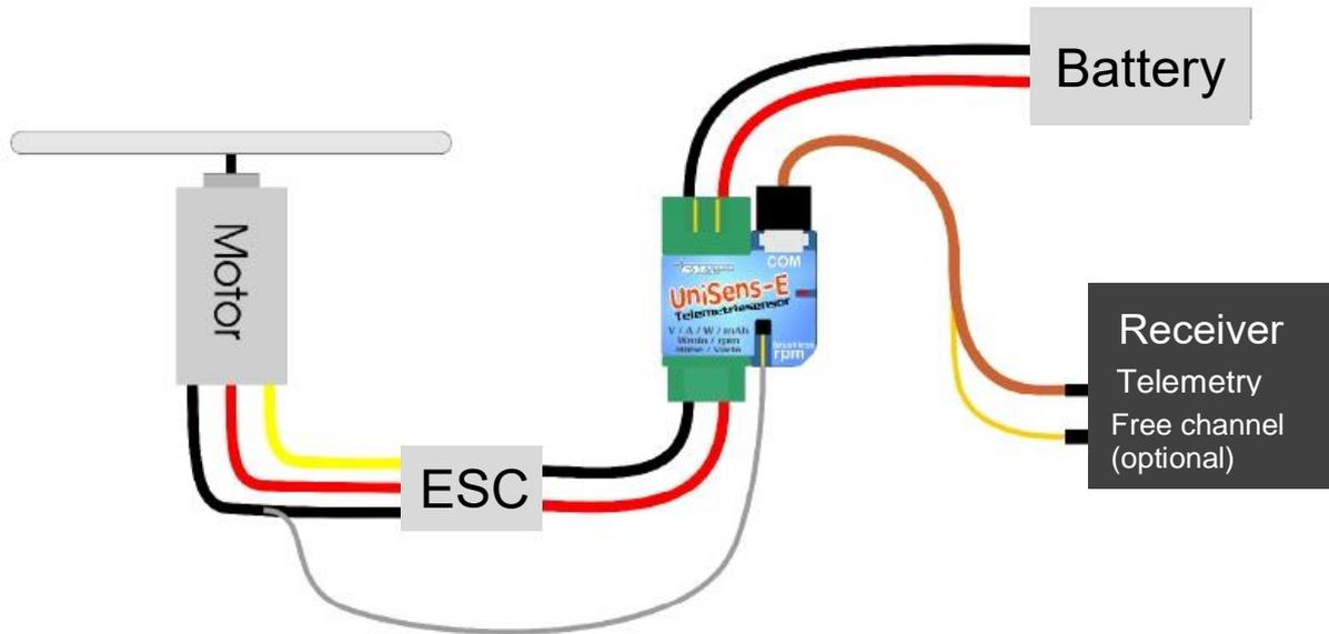
The UniSens-E is placed directly between the battery and controller. Since the UniSens-E is available with various connector systems, normally no soldering is required.
