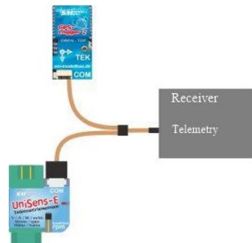
For Robbe / Futaba S.BUS2, JR DMSS, FrSky and Spektrum the COM interface of the GPS logger is not available.
