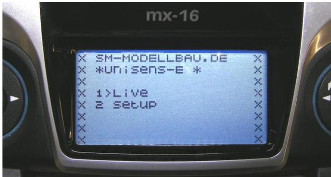
Operation is done with the right touchpad on the transmitter. Structure and content are identical to the screens of the UniDisplay, see also Chapter 9. Here you can also set all the alarms, the beep from the transmitter or the voice output.
