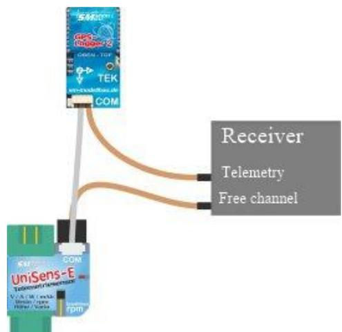
In Jeti Duplex (not EX!) The telemetry data from the UniSens-E is passed from the GPS logger to the receiver. That allows you to avoid the otherwise necessary Jeti E4 expander.
