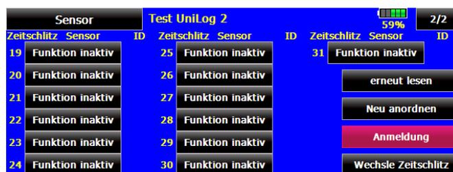
To be able to represent all values the menu item "Login" on the transmitter must necessarily be called 6 times. The message "OK" will appear four times, at the fifth time the message is "sensor already exists".
