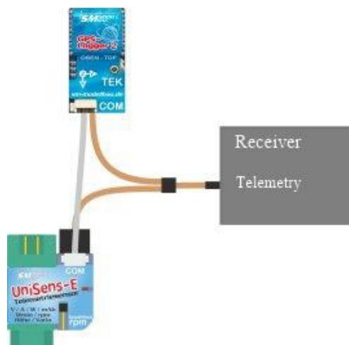
With HoTT and M-Link the UniSens-E and Gps-Logger are connected to the telemetry port in parallel with a simple V cable. Even more sensors can be connected by a V cable.
