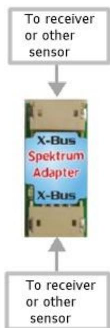
The Spektrum Adapter has a servo connector for the telemetry cable from UniSens-E as well as two X-Bus connections. An X-Bus connector is connected to the X-Bus of the receiver with the enclosed cable. On the second X-Bus connector another Spektrum compatible sensor can then be used. The two X-bus connectors are identical and can be exchanged as desired.
